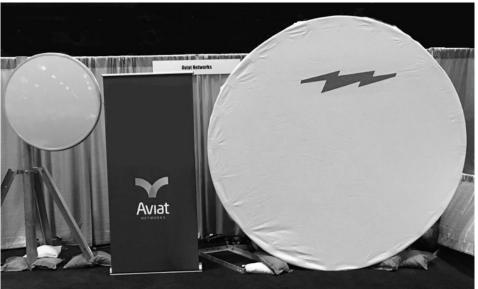
Figure 2. Size comparison between a 1.2m (4ft) and 2.5m (8ft) antenna
