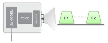
Figure 5. Aviat WTM 4100 single header (1x Tx/Rx) with A2C architecture
