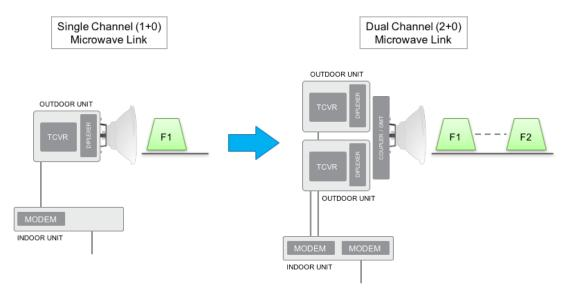
Figure 3. Doubling capacity of a 1+0 link with 2+0 Dual Channel
