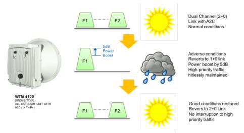
Figure 7. A2C 'adaptive' link operation
