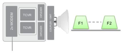
Figure 4. Double-Header (2x Tx/Rx) radio architecture
