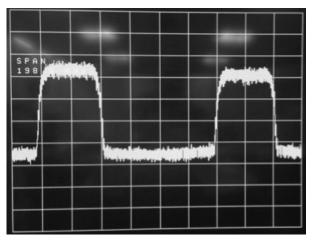
Figure 6. A2C Spectrum for 18 GHz A2C link, 4096QAM, 2x80 MHz channels, supporting total throughput of 1.5 Gbit/s
